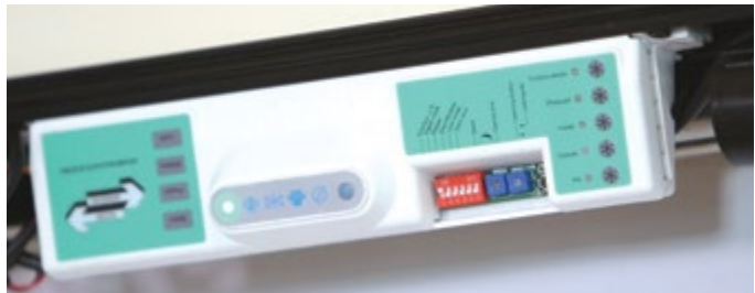
Inside View of the Controller
